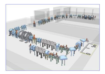
Radionuclides are produced inside a thick target using proton and alpha particle beams from existing room temperature cyclotron at VECC. The radionuclides diffusing out from the thick target will be ionized in the integrated target-ionsource and then it will be subsequently accelerated using series of LINAC to the desired final energy of about 4 MeV/u.
