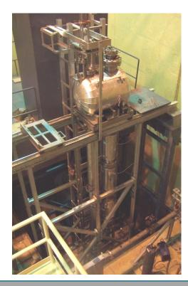
DAE has taken up a comprehensive R&D programme to develop Accelerator Driven Subcritical reactors. One of the key components that have to be developed is the very high intensity neutron spallation target. These targets will be based on heavy density liquid metals like Lead-Bismuth-Eutectic (LBE) alloy. Many issues are required to be studied, which include thermal-hydraulics, corrosion, radiation damage, radiotoxic etc.
