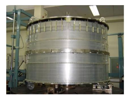
One of the major component of this cyclotron is the super conducting magnet coil which produces very high magnetic field required for rotating high energy charge particles. The magnet coil of the Superconducting Cyclotron is immersed in liquid Helium (4.2K) in a specially built stainless steel Cryostat.
