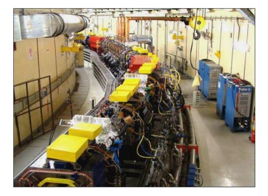
Electrons are accelerated to 2.5GeV using RF source and confined in a circular orbit using bending magnets. The intense low energy synchrotron radiation emitted during bending of the electrons is trapped through beamlines for carrying out R&D experiments.
