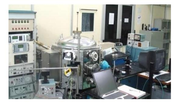
**150 TW Ti- Sapphire Laser:** 150 TW Ti- Sapphire Laser is under operation at RRCAT. At ultra-high intensities using ultra short (femto second) laser pulses, the laser intensity can go more than 10<sup>18</sup> W/cm2.
